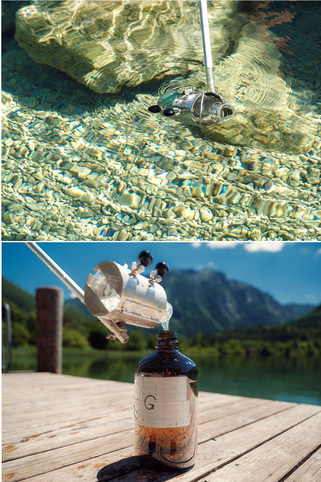
Figure 2: sampling equipment identical to that used in the current investigation (photographed during an earlier study in Austria in 2023), showing sample pole, 500ml sampling bottle and 2.9 litre composite sample container (Winchester)
