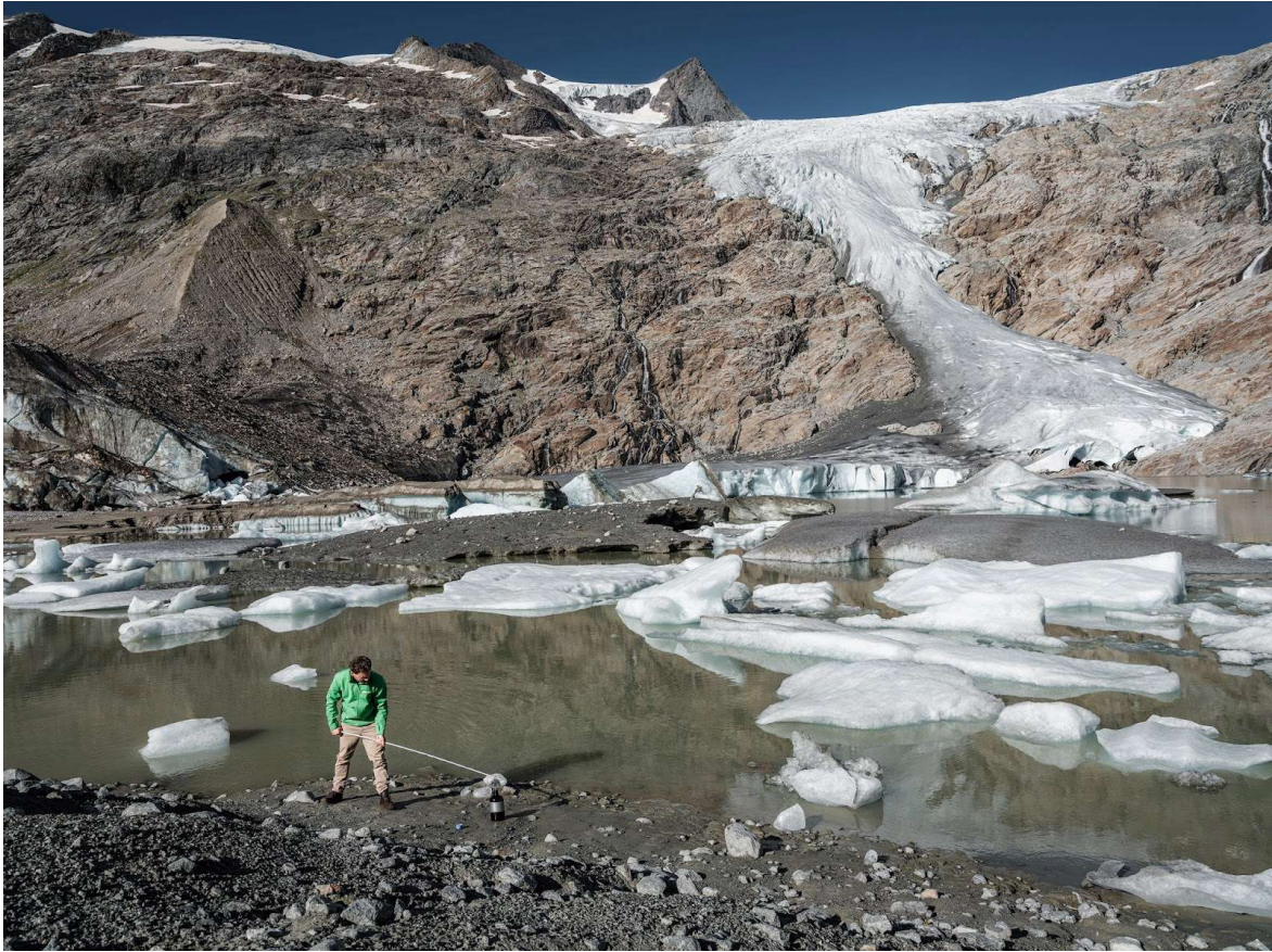
Figure 3: collecting a composite surface water sample beneath the Schlattenkees glacier 'tongue' (Lake Osttirol) during the current investigation, illustrating the measures taken to avoid contamination of the sample during collection (incl. use of long steel sampling pole to hold bottle well away from sample taker, minimal personnel accessing the lake shore itself, washing the outer surfaces of the sample bottles with lake water before opening them and collecting the composite sample).
