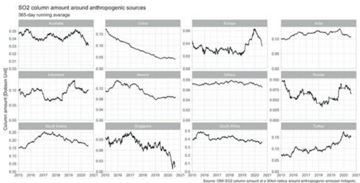
Figure 23: The 2015–2020 SO 2 column amounts within 50km of anthropogenic sources in countries that have large emissions. 365-day running average. ‘Others’ refers to all other countries combined. Data source: OMI.
