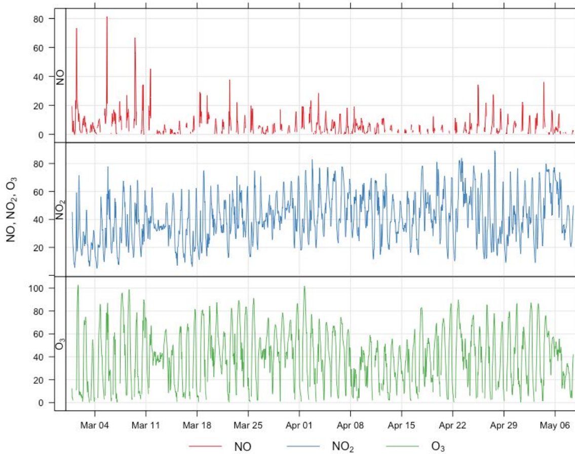
Figure 6: Concentration of NO (Red), NO 2 (Blue) and O 3 (Green) measured by the AQMesh ( \mu\text{g}/\text{m}^3 )
