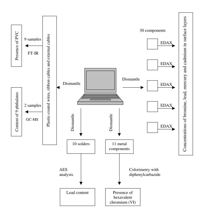
Figure 1. Dismantling of the laptop's components and their analysis
